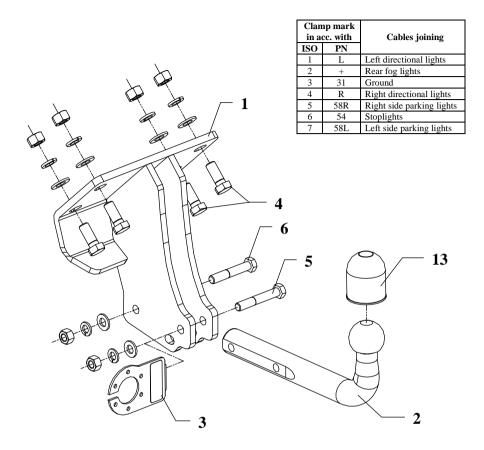
This towing hitch is designed to assembly in following cars: **MERCEDES JEEP 230-300 GE, 250 – 300 GD** produced since 1990, catalogue no. **D25** and is prepared to tow trailers max total weight **3500 kg** and max vertical mass **120 kg**.
